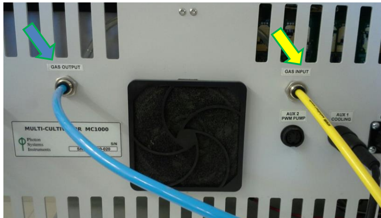
Fig 11. Rear panel of MC 1000 version with gas/air mixing module. Note the gas inlet from Gas Mixing Unit in yellow and gas outlet connector bringing the desired air composition to the humidifier bottle.
