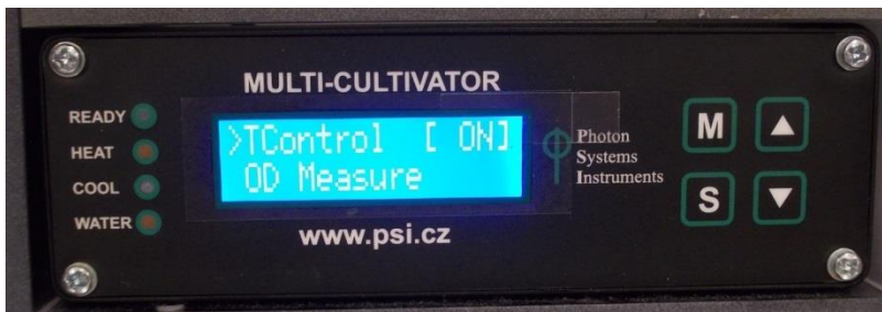
Fig. 9 Display of the MC 1000 control unit when Cooling Unit AC-625 is operating.
