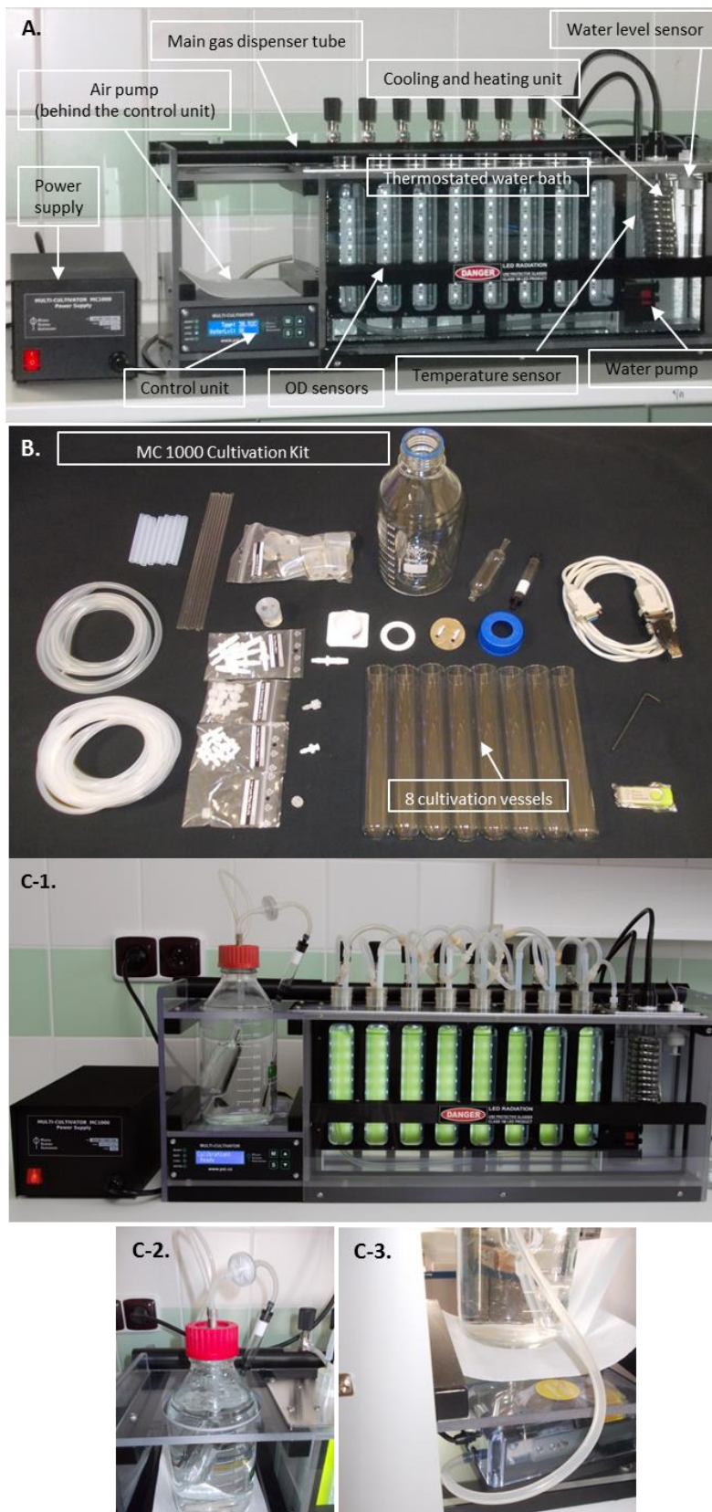
Fig 1. Components of the MC 1000-OD device. A) Front view of the MC 1000-OD. B) Components of the MC 1000 Cultivation Kit. C-1) View of fully assembled and operating MC 1000-OD device. C-2) detail of humidifier bottle set-up is shown. C-3) Detail of air pump connection is shown.
