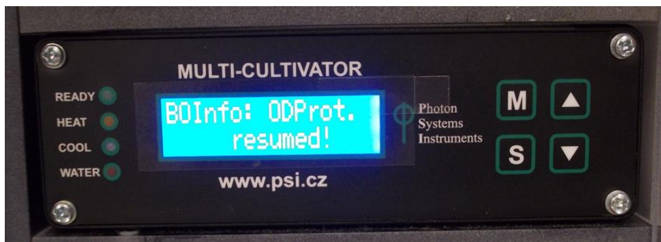
Fig. 26 Control unit display after OD protocol was resumed following MC 1000-OD power outage.
