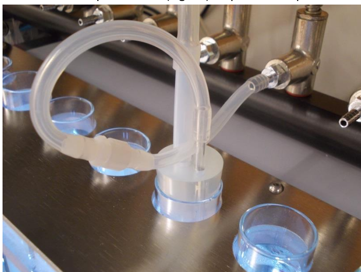
Fig 18. Connection of the cultivation vessel to the main gas dispenser tube.
