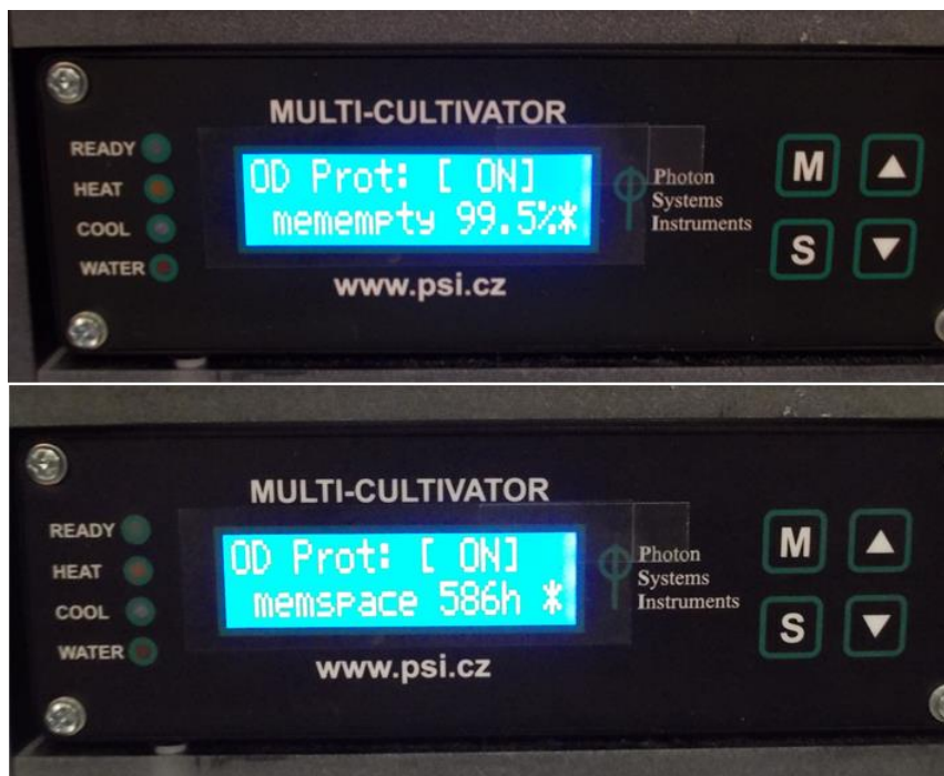
Fig 20. Control unit display with remaining memory space in % and in hours is shown.
